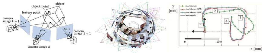
**Fig. 1** Estimation of pose of sensors onboard moving vehicle. Trajectory of moving vehicle is estimated based on sensor locations in current and previous frames. Localization accuracy depends on the type of sensor and type of features computed from the data stream.
