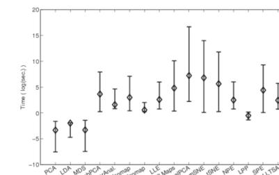
The computational time for all the techniques is displayed on a log scale. The error bars denote the variation across categories, showing the minimum and maximum time utilized. The traditional linear methods PCA, LDA, and MDS are the fastest. Importantly, LPP with the best entropic performance is also faster than other non-linear methods.
